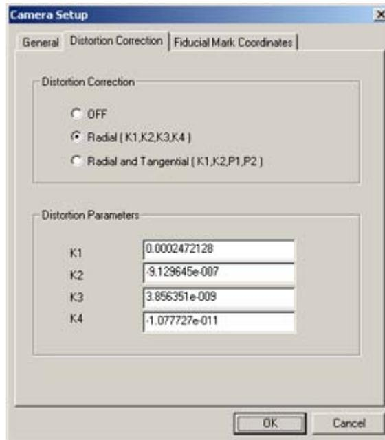
On this page you can enter the settings for correcting lens distortion.
