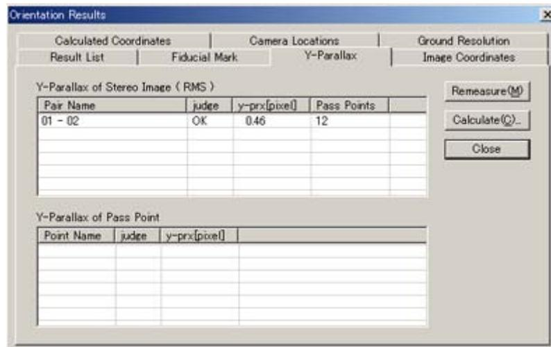
The vertical parallax (y-parallax) of all pass points can be checked here. This page is used when specifying fiducial marks of poor accuracies.
