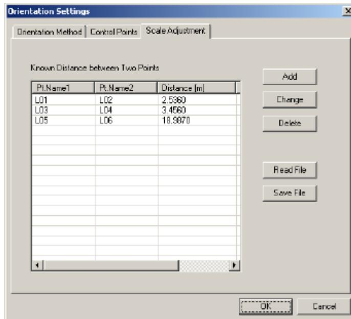
Register a distance between two known points which to be used for the Orientation calculation.
