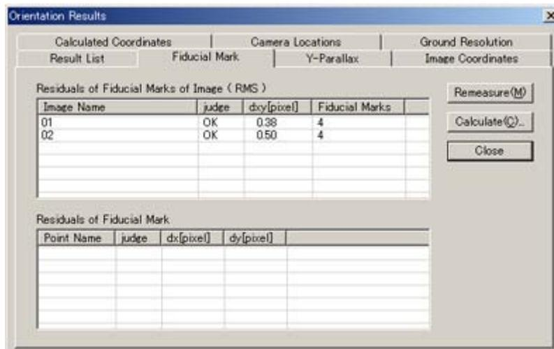
Residual errors of all fiducial marks can be checked here.
