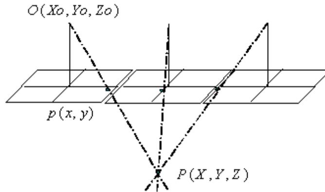
In the bundle adjustment method, the position and angles of all cameras and 3D coordinates of all pass points are determined at the same time. Also, using coordinates of the ground control point, errors are adjusted on the whole. The bundle adjustment is evaluated as image measurement method with the highest accuracy.
