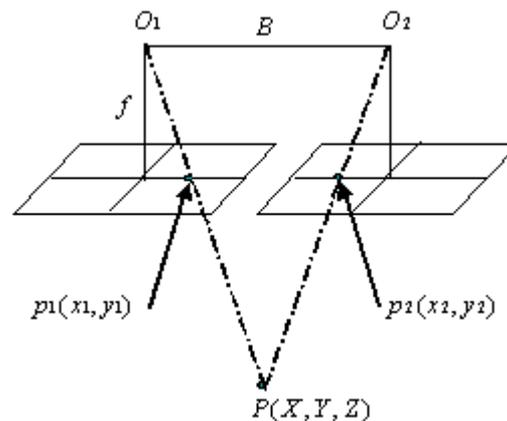
In the stereo image method, the object is photographed from different positions (right and left), and 3D measurement is done using the overlapped portions. By the principle of triangulation, 3D coordinates of the object are determined from corresponding points of the right and left images.
