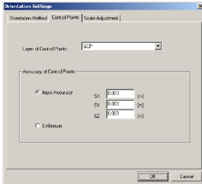
Enter coordinates of the Control Point to be used for the Orientation calculation. To use this Control Point in the Orientation calculation, the same point on the Image to be specified.
