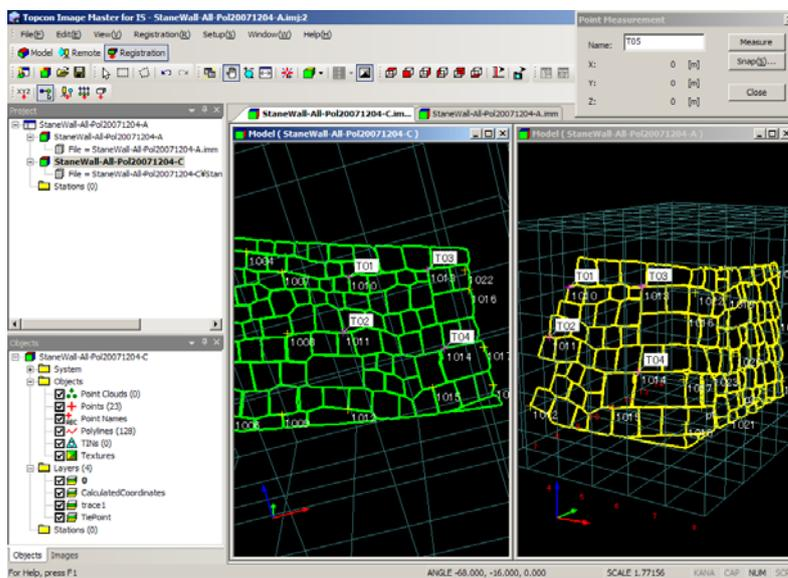
When the tie point is measured, and registration is calculated, two data is connected as shown in the figure below.
